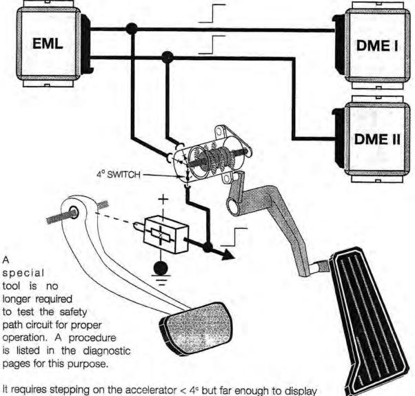
an off idle condition. With this displayed on the DIS screen, stepping on the brake pedal will display the decel fuel cut off request to the DME.
