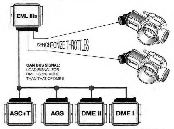
The EML control module processes the load signals from the two DME control modules. If a difference exists, the EML will adjust the DK motors to achieve equal air throughput on both banks.
