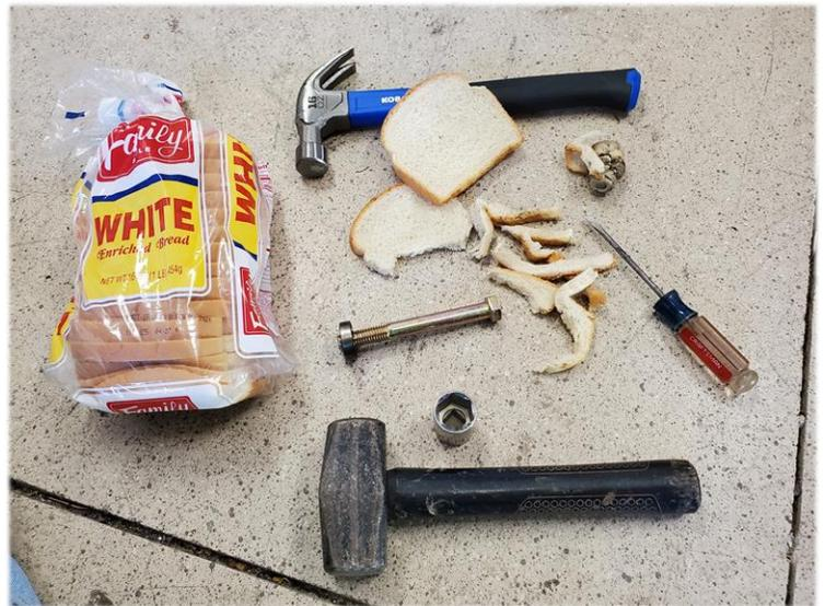
In went the new pilot bearing, flywheel, clutch, pressure plate and all the trimmings followed by new seals, and the transmission reinstalled. All in all, it took maybe 5 or 6 minutes to remove the Pilot Bearing. And it would probably have been less had I not
