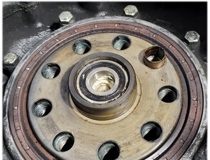
So, Pilot Bearing in pocket, I set off to Lowes to buy a bolt or wooden dowel that fits as closely as possible to the internal diameter of the Pilot Bearing as recommended in the Youtube video. After arriving home, under the car I go, and proceed to "feed" my car bread. And just like a baby that does not want to eat, I "force feed" my CSI bread, then beat it into place with the
