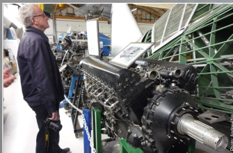
Glen admiring a Rolls-Royce Merlin (27 litre, V-12) engine.
