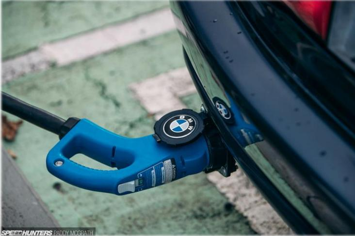
The largest giveaway is the recently added CHAdeMO fast charging port which resides where the passenger side exhaust tip once lived. This is in addition to the slower Tesla 10kW charging port which hides behind the factory fuel filler cap. If you get down on your knees and look under the rear, it is difficult to miss the Tesla unit, providing you know what it is in the first place.
