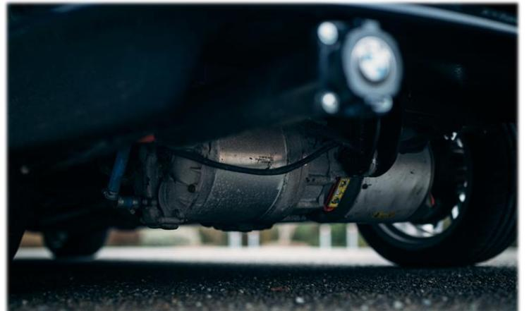
It was always Damien’s intention to convert the 8 Series, and not long after arriving home he had removed the 4.4-litre M62B44. In its place went a Siemens 1PV5135 electric motor connected to
