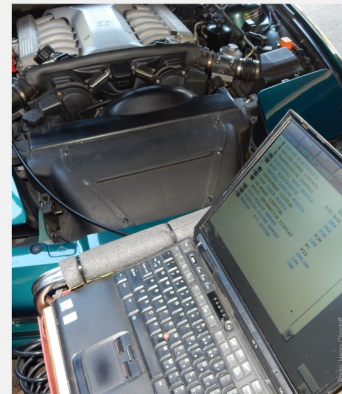
The GT1 reading SRS fault codes on Vic's E31.
